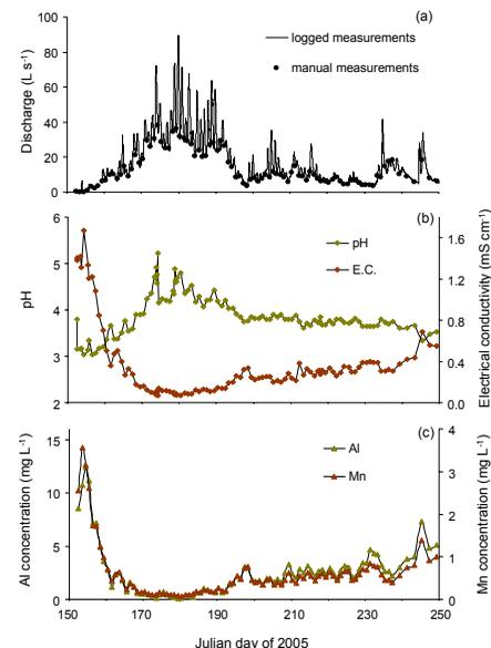
**Figure 1.** Temporal variations in flow rate and dissolved runoff chemistry measured at the location of the weir. (a) Flow rate of runoff; (b) pH and electrical conductivity and (c) Al and Mn concentrations.
