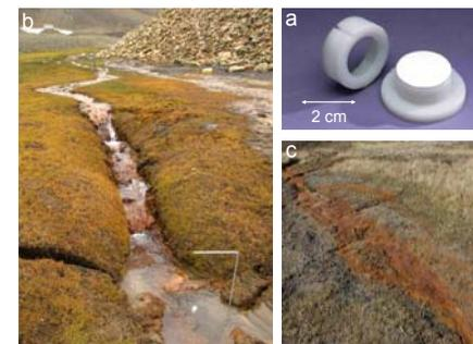
**Figure 4.** (a) Labile and potentially 'bioavailable' Al and Mn concentrations in the drainage water were measured using the in situ speciation technique of diffusive gradients in thin films (DGT). (b) A DGT sampler hangs suspended from a rod in a small runoff stream. (c) Vegetation damage in the area down-stream from the waste pile (c) is presumably mainly due to high Al and Mn concentrations in the runoff as well as Fe(II) precipitates.
