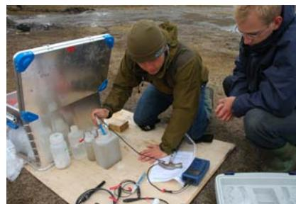
**Figure 3.** Fieldwork during 2005 and 2006 included daily water sampling and in situ measurements of pH, electrical conductivity, dissolved oxygen, and redox potential.
